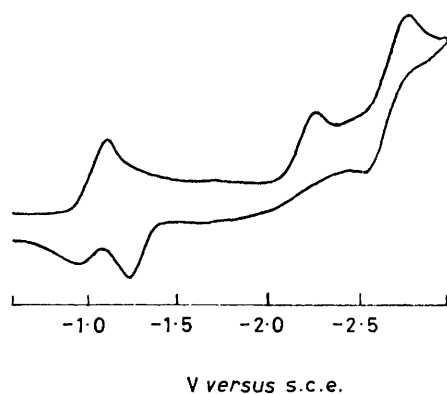
FIGURE 5 Cyclic voltammogram of 1 × 10 -3 mol dm -3 [Co(C 2 F 5 )(salen)] in thf (0.1 mol dm -3 [NBu 4 ][ClO 4 ]). Hanging mercury-drop electrode, scan rate 10 V s -1 , potential range -0.58 to -2.98 V versus s.c.e.
